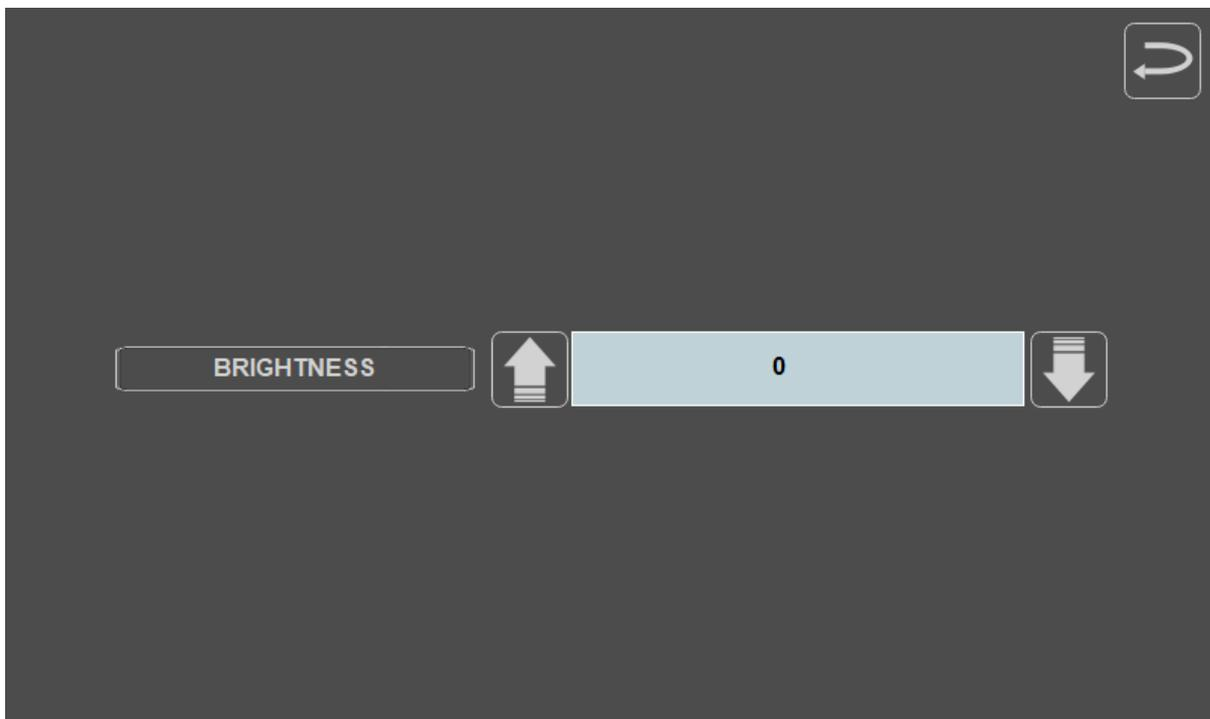
Use the “UP ARROW” or “DOWN ARROW” keys to adjust the light intensity of the display.
