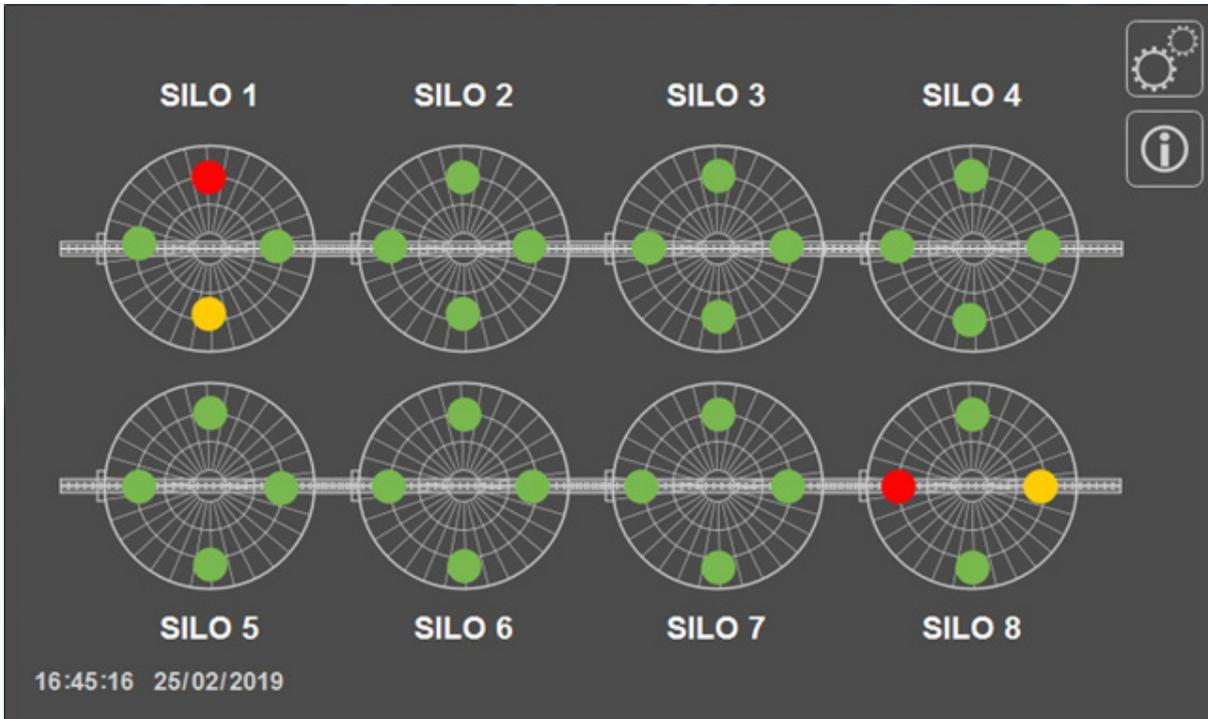
From the HOME page it is possible to access the silo temperature display page (by pressing the MENU button), the display page of the values read by the single probe (by pressing on the single green/yellow/red colored circle), the AGRITHERMT60/ configuration page T60 PLUS (by pressing the “SETUP” button) and system information (by pressing the “INFO” button).
