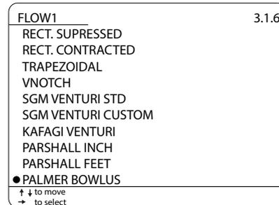
Enter the inner diameter of the pipe were the Palmer Bowlus is installed. Move the cursor with “RIGHT”, and press “UP” to change the digit. Press “ENTER” to confirm.
