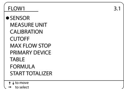
Select the SENSOR\_x installed on channel with "UP" or "DOWN".
