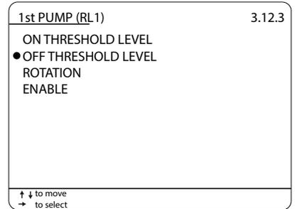
Set in mm the off threshold level value.
