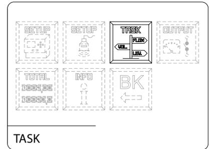
Press “RIGHT” to access the submenu “VOLUME1” or “VOLUME2”, is possible to configure up to 2 volume measurements.
