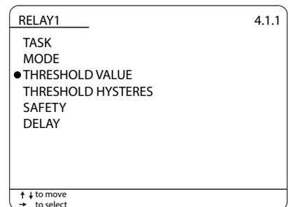
Set the flow threshold value. Move the cursor with "RIGHT" and "UP" to change the digit.
