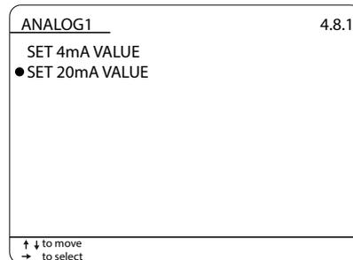
Set in mm the level value corresponding to the 20mA output.
