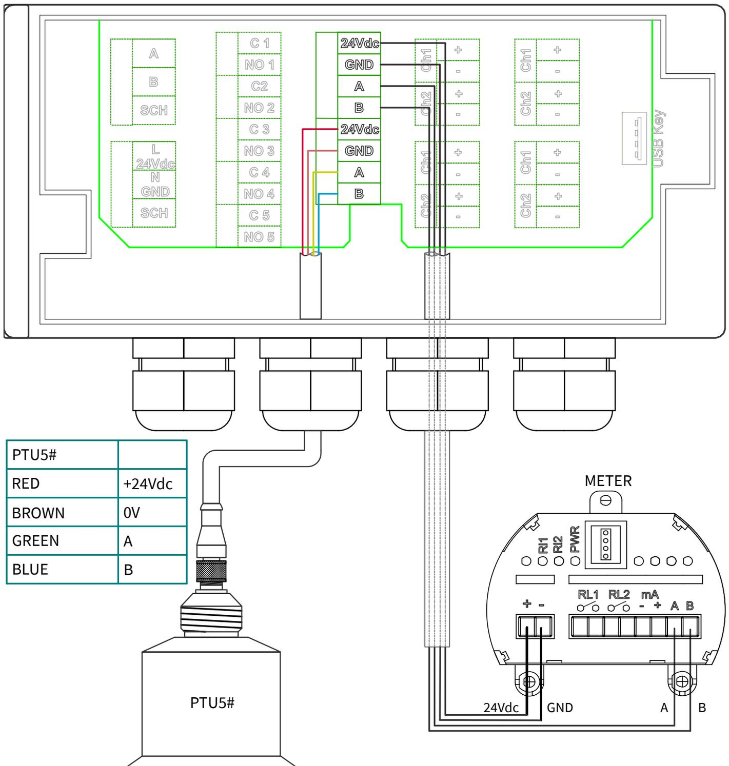
6.3.2 - With more than two ultrasonic sensors SGM LEKTRA, 24Vdc additional power supply is needed
