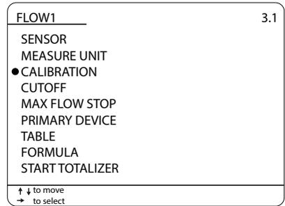
“MAX Q” is the threshold for Max flow beyond which the tot. does not increase. Set the value and confirm with “ENTER”. Disabled function with “0” threshold value.
