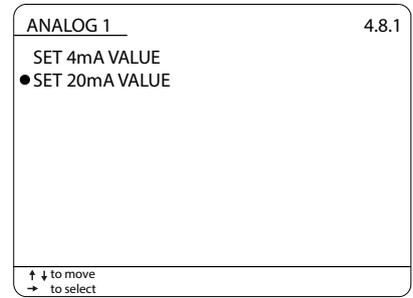
Set in mm the differential level value corresponding to the 20mA output.
