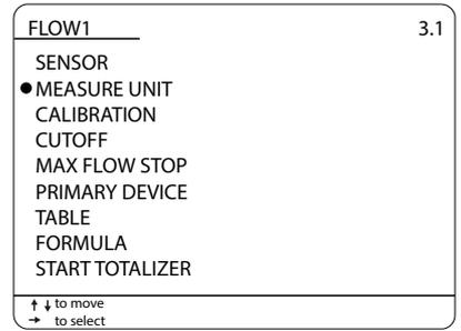
Press “UP” or “DOWN” to select the flow rate measure unit and press “RIGHT” to confirm.
