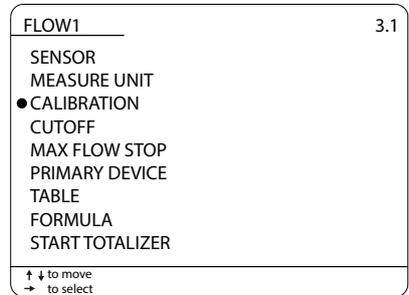
"MAX Q" is the threshold for Max flow beyond which the tot. does not increase. Set the value and confirm with "ENTER". Disabled function with "0" threshold value.
