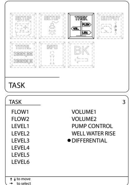
N.B. - Perform the steps described in 10.1.1 and 10.1.2 sections (CALIBRATION) during the “Level difference = 0” real condition, because this condition allows to enter the same “ACTUAL LEVEL” value, automatically obtain the correct 0 setting (UPSTREAM LEVEL - DOWNSTREAM LEVEL = 0)
