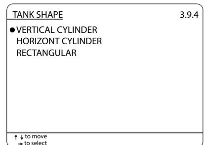
Enter the diameter in mm and, if necessary, the tank/silo conical part
