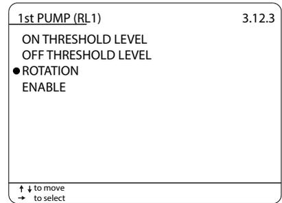
Select “YES” to enter the pump operating cycle in the working times table. The pump that has accumulated the lowest operation time will be turned on for the first. Press “RIGHT” to confirm.
