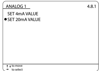
Set in mm the volume value corresponding to the 20mA output.
