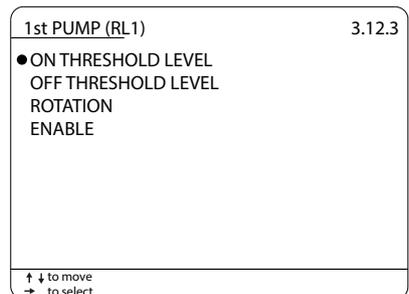
Set in mm the on threshold level value.
