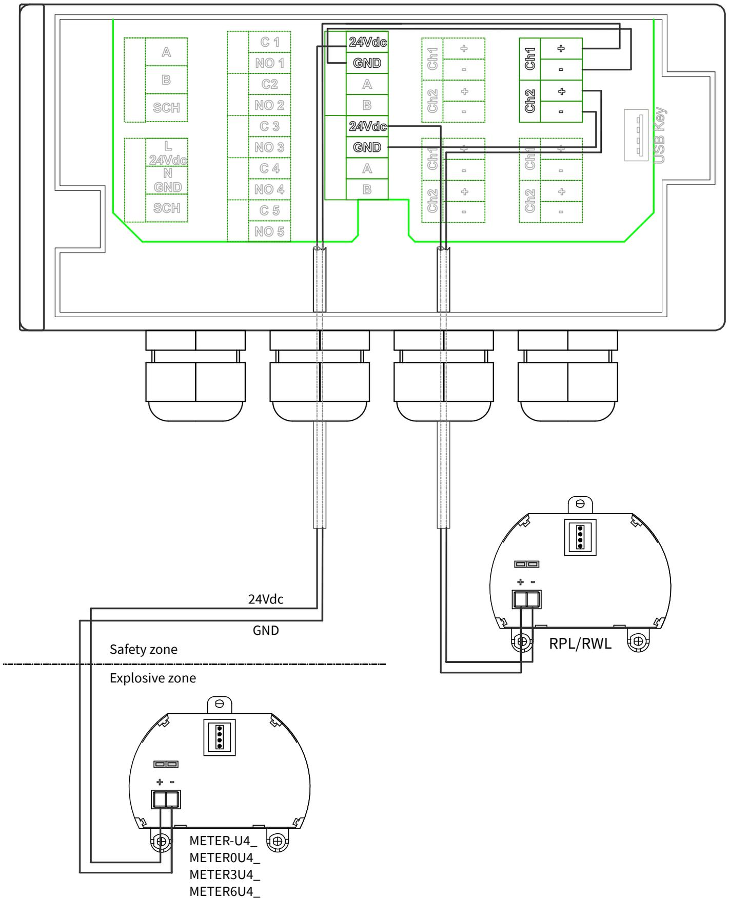
6.3.4 - SGM LEKTRA hydrostatic head level transmitters connection
