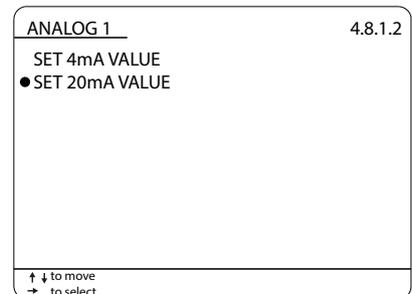
Set the flow rate value corresponding to the 20mA output.
