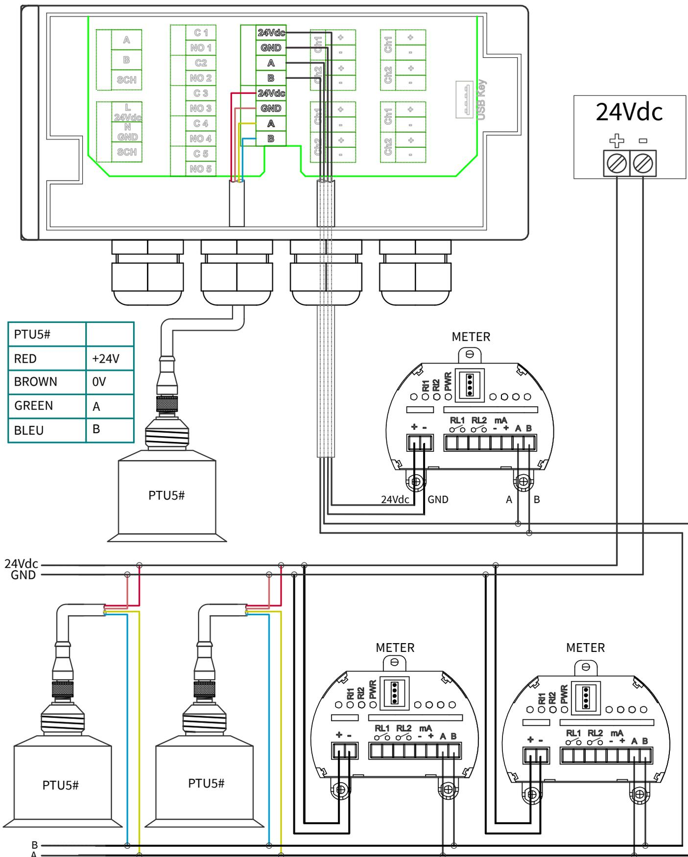
6.3.3 - ATEX certified METER or radar RPL / RWL level transmitters connection
