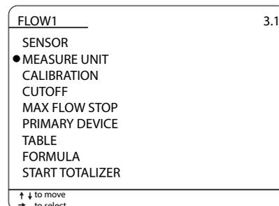
Press “UP” or “DOWN” to select the flow rate measure unit and press “RIGHT” to confirm.
