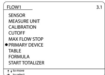
Press "DOWN" to select "RECT. CONTRACTED" and press "RIGHT" to confirm.
