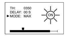
By setting the MODE parameter with the "MAX" option, the RSL200 sensors will work in maximum level alarm mode:
