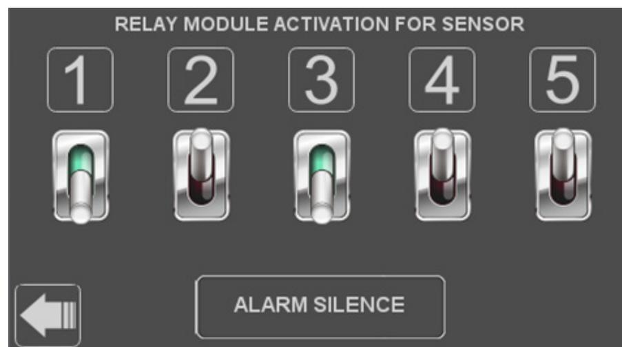
Pressing the “ALARM SILENCE” key forces the relay module to deactivate the alarm signal, which will in any case remain visible on the display on the sensor page.
